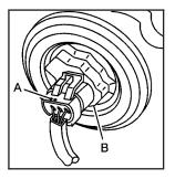
Press the clip (A) on the electrical connector when replacing the low-beam or high-beam bulb, then pull it straight off. Turn the bulb retaining ring (B) counterclockwise to remove it and then pull the bulb assembly straight out.
